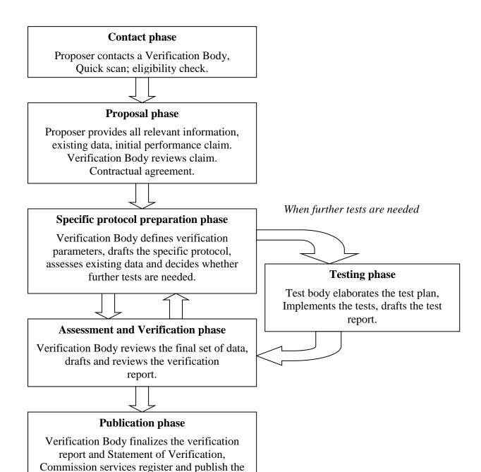
Figure 2: Phases of the EU ETV pilot programme verification procedure
